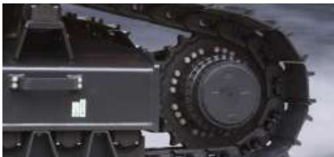
Travel motor Running drive force improved with the efficiency improvement of the running device, its performance is excellent at a slope or swampy area.
