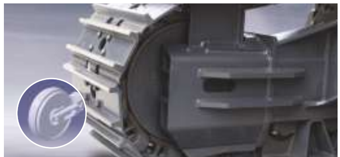
Integrated track spring and idler The track spring and the idler have been joined directly to achieve high durability and improved maintenance convenience.
