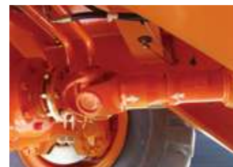
Transmission shaft: Apply reinforced transmission shaft and self-locking nuts are used as the connecting bolts of the transmission shaft so as to improve the durability of transmission system.
