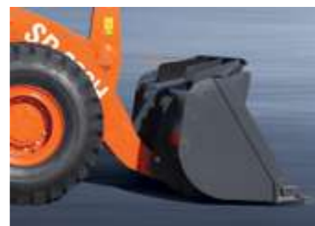
Wear-resistant materials are used for the bucket, and robust design applied upper parts of the bucket, which may effectively prevent the deformation of the bucket caused by stones and other falling objects.
