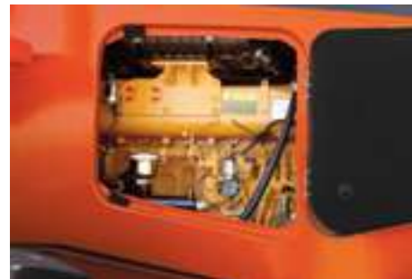
Maintenance windows have been added to each side of the engine hood, thus making daily oil inspection and maintenance works quicker and more convenient.
