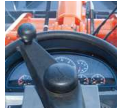
The interior decoration in the cab is upscale : FRP-ABS materials are used for dash board and console and striae treatment is applied to the surface, which is high-grade and durable.
