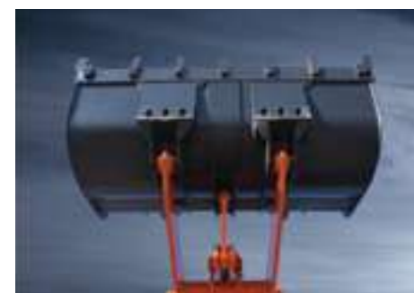
The diameter of the hinge pin in the 6 operating devices is 5-10mm larger than the level of the industry. High wear-resistant materials are used for pin sleeves so that the durability of working device is stronger and the residual value of second-hand equipment is higher after being coated with MoS2 and processed with a special heat treatment process.
