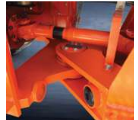
Hinge Limit DISD loader adopts a new part - the nylon hinge limit block. It has stronger durability, no noise caused by impact and reduces the driver's fatigue.
