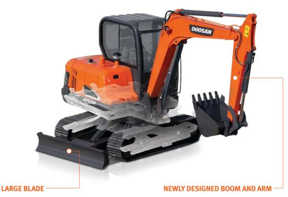
Large blade with increased soil removal capacity implemented by high-durability material and wide-area design.
