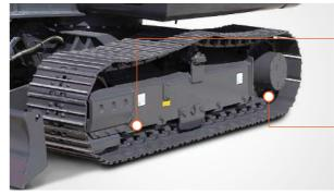
The track roller attachment point was shifted from lower to middle portion to improve undercarriage stability and structural rigidity of the chassis.
