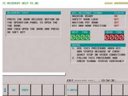
ATC recovery help It makes operator recovery of the ATC from alarm status easier.
