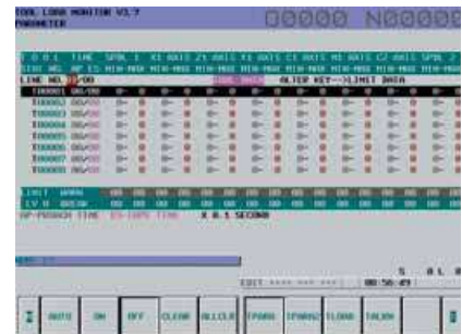
Tool load monitor opt. The axis and spindle load in cutting are monitored which minimises damage to the tool.
