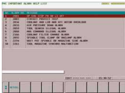
Alarm guidance Recovery method for important alarms is displayed on the screen.
