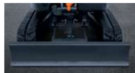
Dozer Blade Welded, unitized blade provides durability even under harsh working conditions 1,700 mm x 350 mm (5'7" x 1'2")
