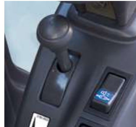
E/G Control Lever The engine control lever is placed in a very convenient location easily accessible by the operator to easily control the engine speed.
