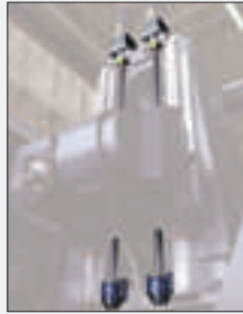
Applying a Dual ball screws on the Y-axis to improve rigidity.
