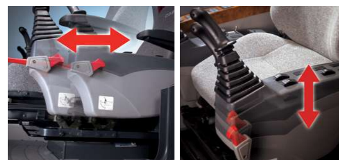
Comfortable 2-stage sliding seat Control stand (Telescopic Function)
