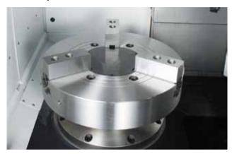
The cartridge type spindle with A2#8 spindle nose assures high capability and easy of maintenance. Especially rigid coupled bearing assembly is to support heavy weight workpiece and reduces thermal growth in long run operation.
