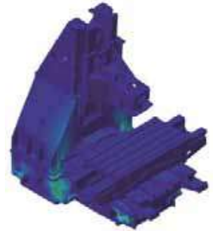
• FEM analysis used to design a stable body. ( FEM : Finite Elements Method )
